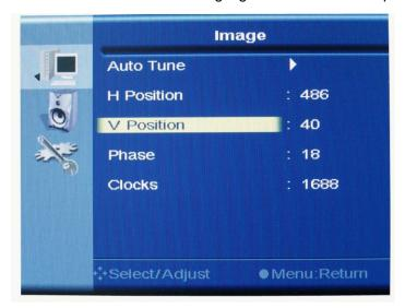
b. Press " $_{\triangle}$ " or " $_{\nabla}$ " to move the vertical position of OSD . Then press "1" to confirm the adjustment and back to Image menu.
